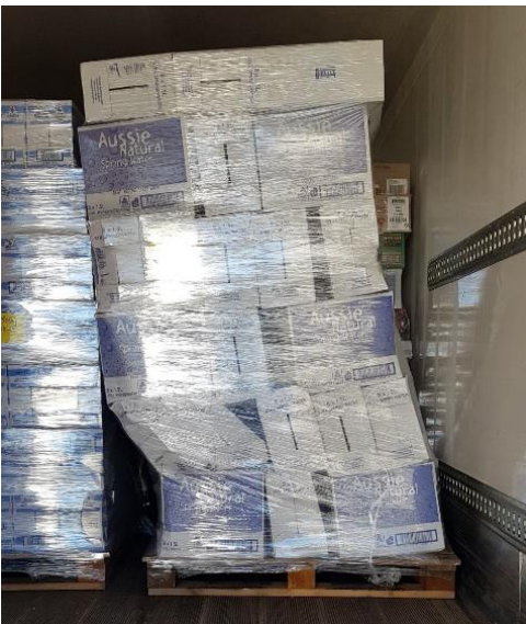
Example: Poorly wrapped pallet. Stretch wrap needs to be at a high tension and needs to be several layers (not single layered). The pallets here have insufficient layers of stretch wrap which has resulted in the goods shifting during transport and falling over.
