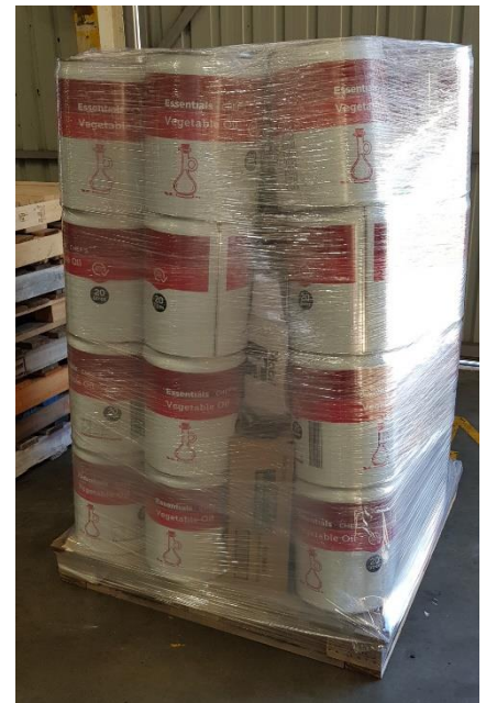
Example: Poorly stacked pallet. Pallet is stacked with spaces between the tins and wrapped too tight resulting in the tins collapsing at the top and all coming together.
