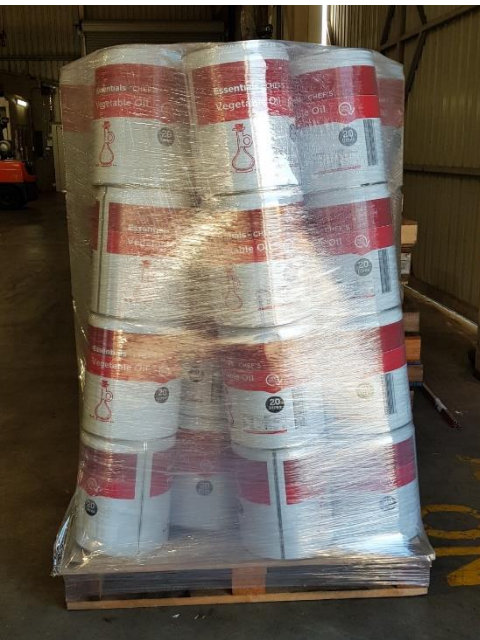
Example: Poorly stacked pallet. Pallet is stacked with spaces between the tins and wrapped too tight resulting in the tins collapsing at the top and all coming together.
