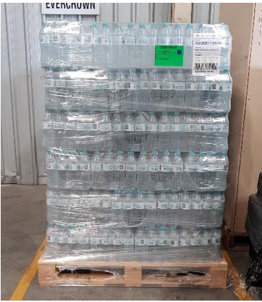
Example: Well palletised goods. The additional use of strapping and cardboard edges also improves the stability of a stretch wrapped pallet in transit.
